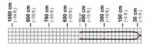
Typical beam pattern for 30cm target move left and right with the board parallel to the sensor face.
